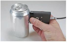
Note: Flex 20 measurement area 6x6 mm. With optional adapters 2x2 mm & 4x4 mm measurement area.
