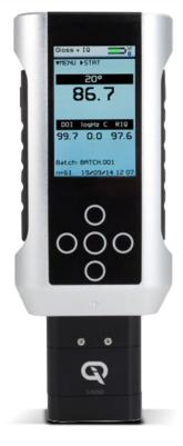
The Rhopoint IQ FLEX 20/60 brings appearance measurement to a higher level, specifically designed for difficult surfaces or small parts. The small footprint of the IQ FLEX 20/60 sensor makes for easier measurement of curved surfaces and difficult to reach areas when compared to a conventional glossmeter.
